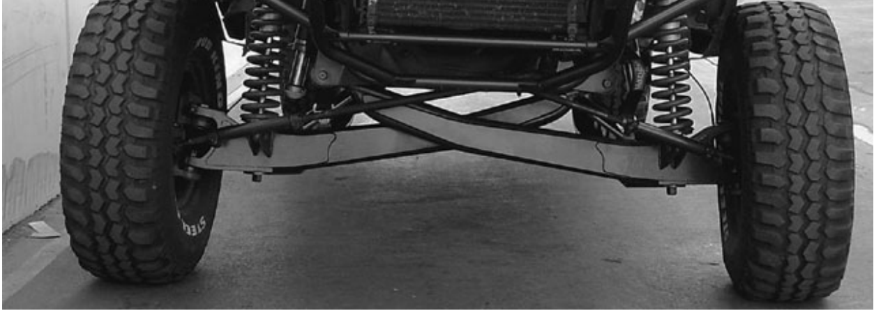
Figure 3: I-Beam Suspension Design [3]
