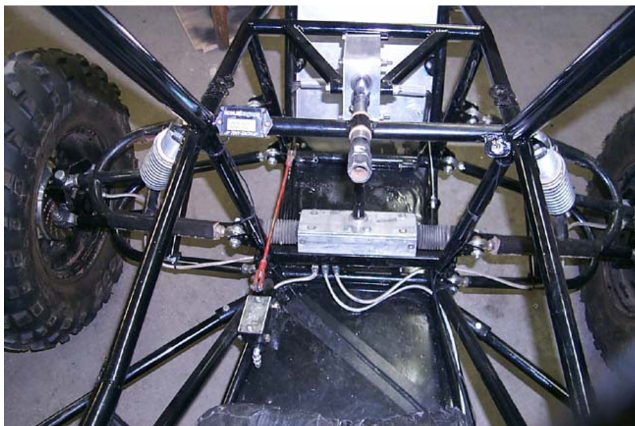
Figure 8: Back Mounted Rack and Pinion [8]
