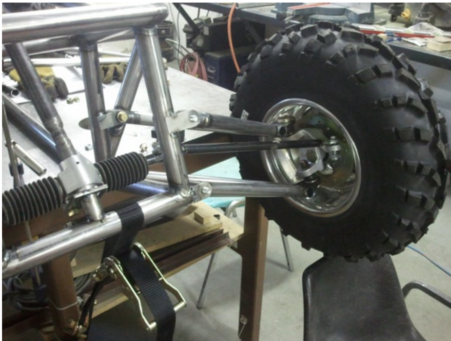
Figure 9: Front Mounted Rack and Pinion [9]
