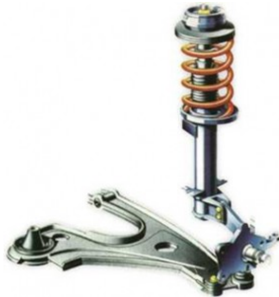
Figure 2: MacPherson Suspension Design [2]
